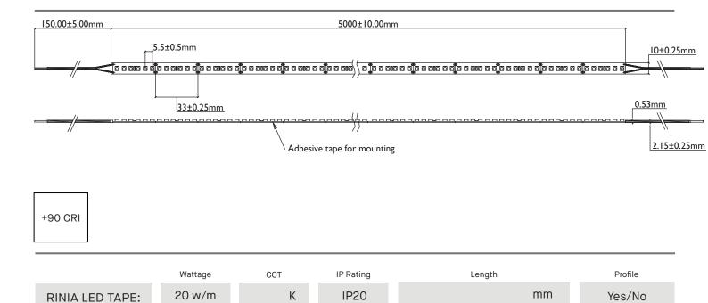
Rinia LED tapes provide an extensive range suitable for residential and commercial applications. Binned to two to three Macadam steps, the Rinia tape provides an industry leading quality of light. Supplied in reels to be cut and soldered on site or made to order within custom profiles with end caps and pre-wired tails.
