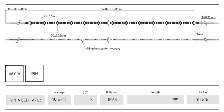
Rinia LED tapes provide an extensive range suitable for residential and commercial applications. Binned to two to three Macadam steps, the Rinia tape provides an industry leading quality of light. Supplied in reels to be cut and soldered on site or made to order within custom profiles with end caps and pre-wired tails.
