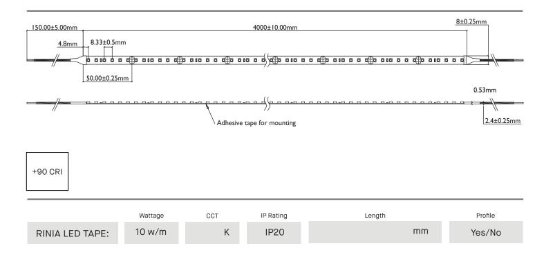
Rinia LED tapes provide an extensive range suitable for residential and commercial applications. Binned to two to three Macadam steps, the Rinia tape provides an industry leading quality of light. Supplied in reels to be cut and soldered on site or made to order within custom profiles with end caps and pre-wired tails.
