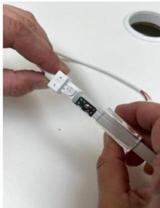
**Step 5:** Place the holding clip in line with the silicone. (The end with the clip facing outwards)
