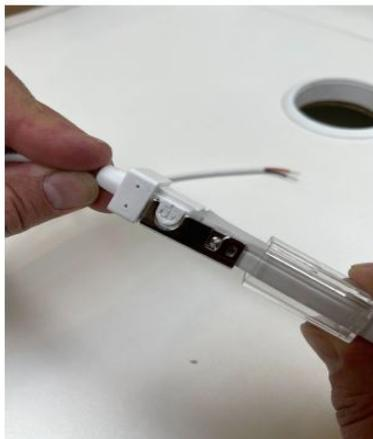
**Step 7:** Press together until clipped in securely.
