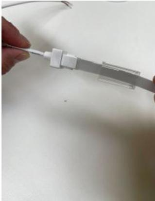
**Step 4:** Place the metal prongs in between the copper and the LED.
