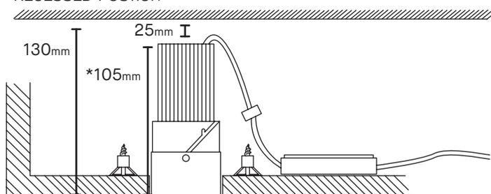
\* For the 1300lm Xicato engine package, add 15mm to these measurements to accommodate a larger heatsink
